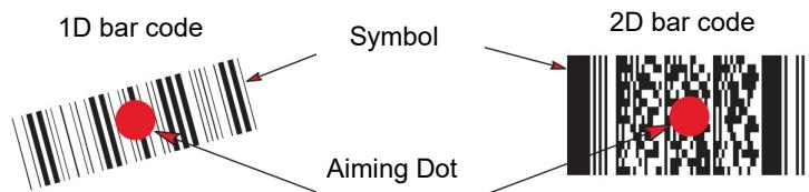
5. Hold the trigger until the digital imager reader beeps, indicating the barcode is successfully decoded.
