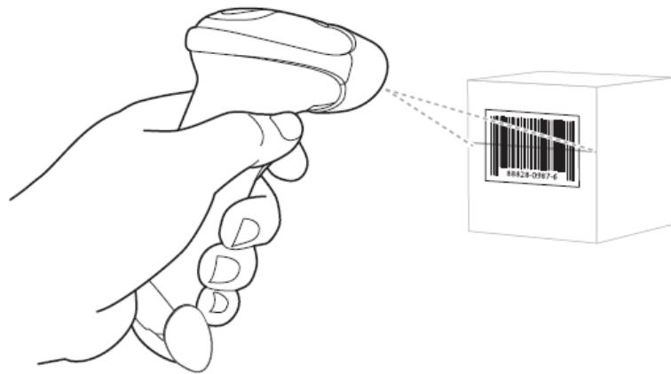
Do not hold the reader directly over the barcode. Laser light reflecting directly back into the reader from the barcode is known as specular reflection. This specular reflection can make decoding difficult. You can tilt the reader up to 55° forward or back and achieve a successful decode.
