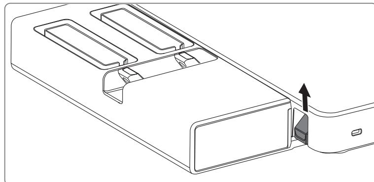
3. Use three screws with the same type only to fix the module to the main unit.
