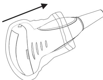
3. Secure the sheath with the enclosed elastic bands.
