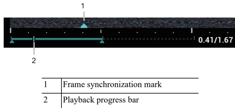
The frame synchronization mark on the time mark of M/PW image indicates the corresponding 2D image and M/PW image. In statuses other than dual live status, you can only review images in the currently active window.
