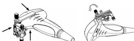
2. Adjust the needle angle to the proper shift as required:
