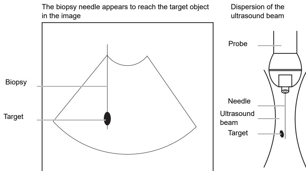
The biopsy needle may not have actually entered the target object even though it appears to have done so in the image. To avoid this, note the points below:
